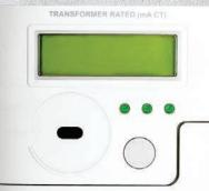
Sieco-Tech RSP-120MA D2EL-3W DIEL-2W Meas Range 120Vac 0.8-100mA 60Hz 3VA - 25 Ct60°C AE-SM: RS1MMA36170904
